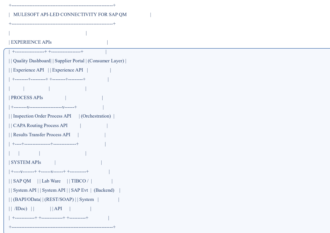
Figure 2: MuleSoft API-Led Connectivity Architecture for SAP QM Integration
